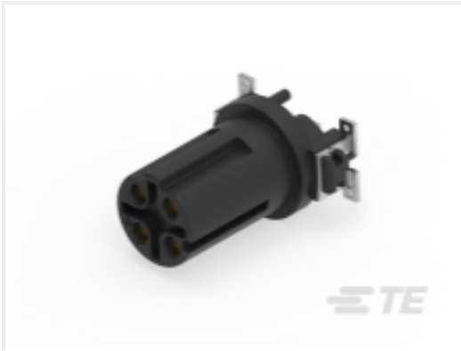
TE Part #454949-E M12 FEMALE, D CODE, 4P, 17MM SMT
