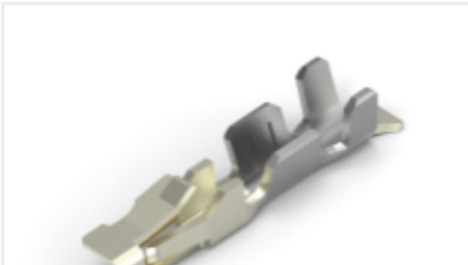
TE Part #5-2316113-6 2MM,REC,CNT,CRIMP,24-28AWG,0.76 UM,LP
