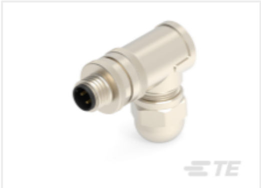
TE Part #T4113512041-000 M12 M, 4P GOLD D_CODE RA SHIELDED PG9
