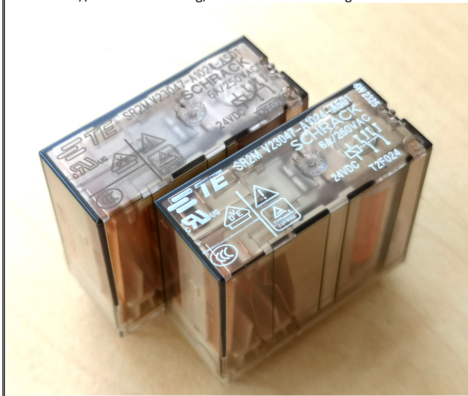
SR2M 2xCO // front: old marking, rear: new laser marking
