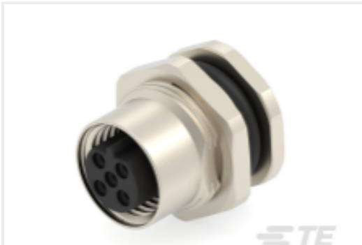
TE Part #T4131412051-000 M12,REAR MOUNT,FEMALE,B,5P, SOLDER WIRE
