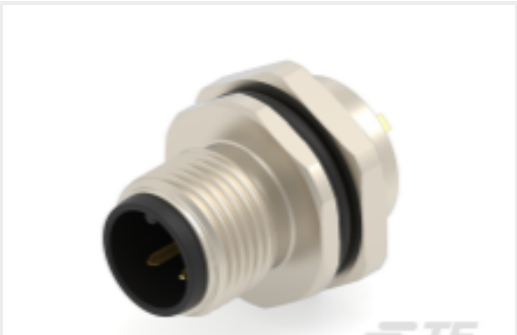
TE Part #T4132012031-000 M12,FRONT MOUNT,MALE,A,3P, SOLDER WIRE
