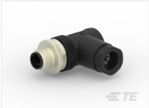
TE Part #T4113002021-000 M12,MALE,RA,A CODE,2P,PG9,GOLD
