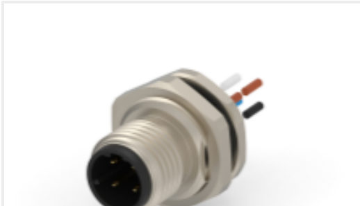
TE Part #T4171010504-001 M12,REAR MOUNTING,MALE,D,4P,0.2 M WIRE
