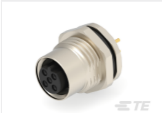
TE Part #T4141412041-000 M12,REAR MOUNTING,FEMALE,B CODE,4P
