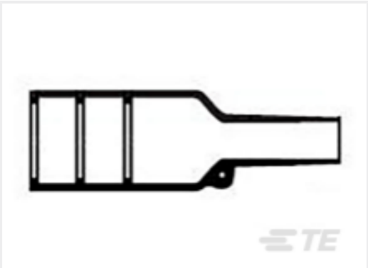
TE Part #CAT-R21-731072 Bulbous Heat Shrink Boots: Lipped, Straight
