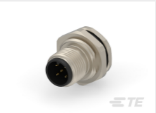
TE Part #T4171010005-001 M12,REAR MOUNTING,MALE,A,5P,0.2 M WIRE
