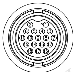
Pin Assignments Front View
