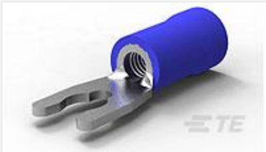
TE Part #52956-2 TERMINAL,PG SPR SPD 16-14 8
